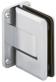
double-action hinges Agita for 8mm glass doors, stainless steel matt up to 60kg leaf weight / 915 mm width (left) up to 100 leaf weight kg / 1200mm width (right)
