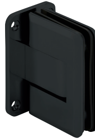
double-action hinges Agita for 8mm glass doors, black up to 60kg leaf weight / 915 mm width (left) up to 100 leaf weight kg / 1200mm width (right)
