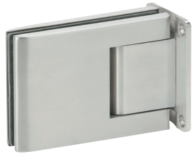
double-action hinges Agita for 8mm glass doors, stainless steel matt up to 60kg leaf weight / 915 mm width (left) up to 100 leaf weight kg / 1200mm width (right)
