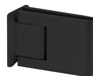
Agita Ultra black.edition Jet black, with hydraulic closing function and adjustable closing speed, max. door leaf weight 100 kg
